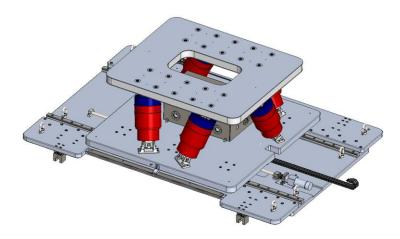
Figure 7. Test Article Positioning System Concept. Credit: Moog, Inc.
