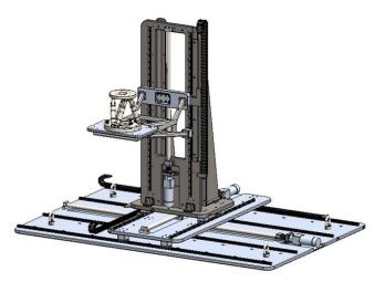
Figure 6. Focal Plane Positioning System Concept. Credit: Moog, Inc.
