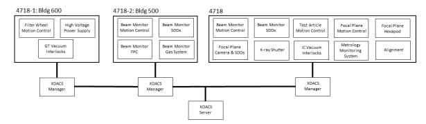
Figure 3. XDACS Block Diagram.
